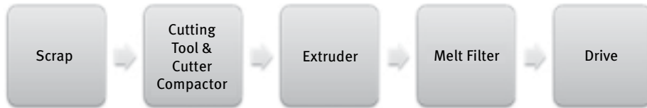
Fig. 9.2: Erema recycling plant concept.
