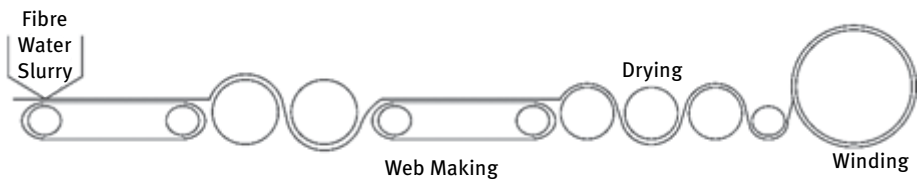
Fig. 4.27: Schematic of wet laid web formation.
